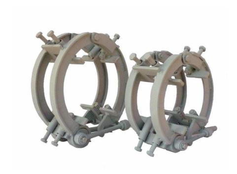
The **MECHANICAL PIPE ALIGNMENT CLAMP** is an equipment for a perfect alignment of pipes, when you need to weld them under optimum conditions. The laying is obtained with an eccentric. The mechanical working of the clamp is suitable for pipes with small diameter and small thickness.
