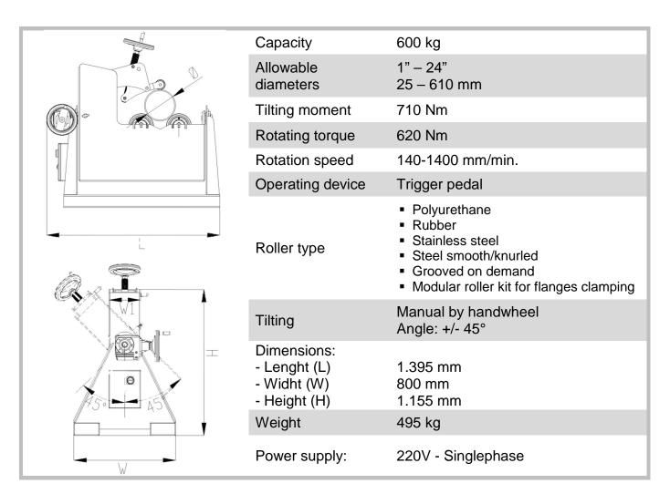
**Tubulu/ 24** is supplied as standard equipment with manual tilting operated by handwheel.
