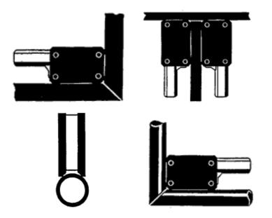
The bearing is studied to to be adapted both to flat surfaces and to round surfaces.
